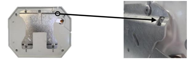
3.1.3.Unscrew the locking screw with Torx T8 tool, **without removing the screw from the plate so as not to lose the seal.**
