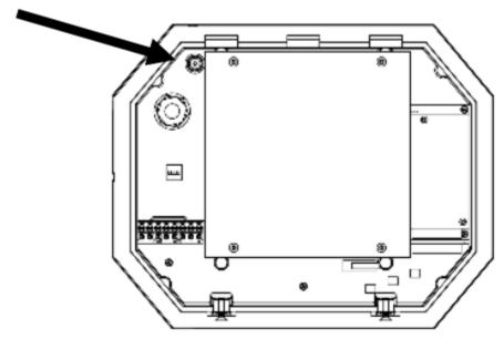
3.1.4.Remove the metal mounting plate by exerting pressure on the metal plate while sliding it. Leave the four mounting screws in place.
