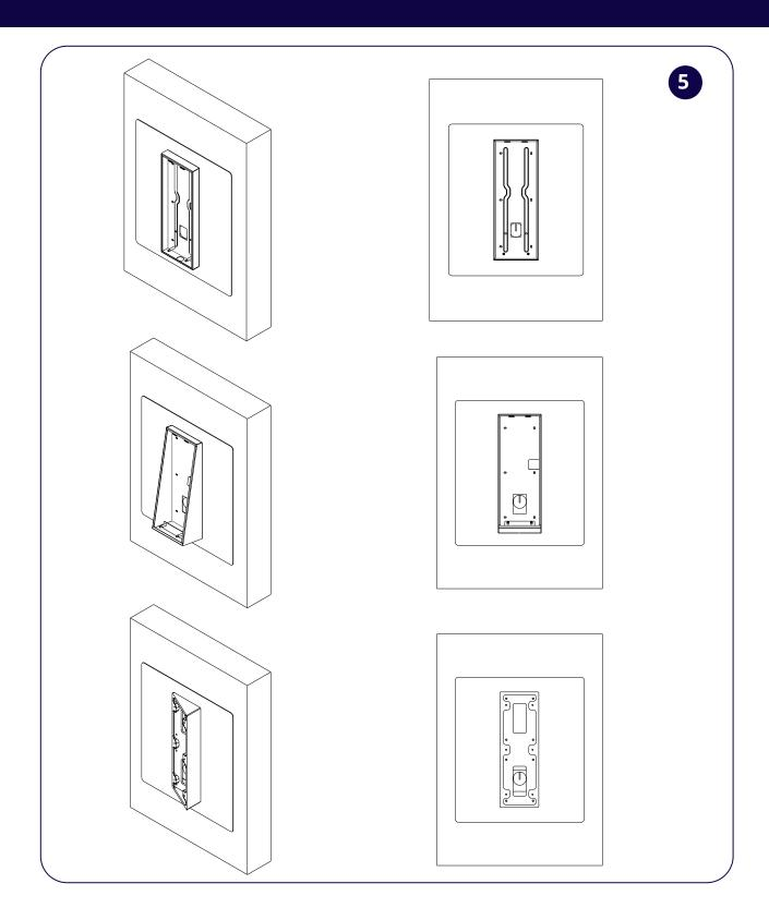
5. Fix the surface back cover with 6 flat wood screws (or 8 for the side angle version) and finish the installation as described in the Swiftreader X installation manual:
