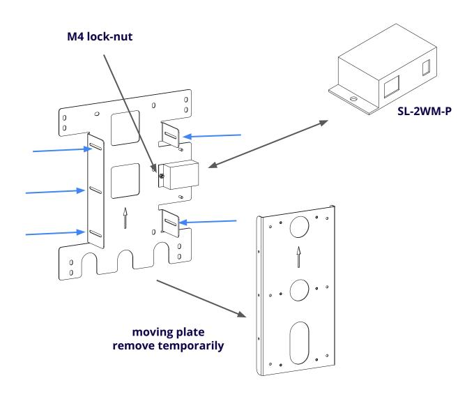
If a 2 wire to PoE+ adapter has to be used, this will positioned to the place shown above. The moving plate would have to be temporarily removed by removing the 5 M4 allen side screws (3 on the left and 2 on the right - positions indicated with the blue arrows) Adapter is fixed in place with one M4 lock nut (provided) Connectors will be facing downwards
